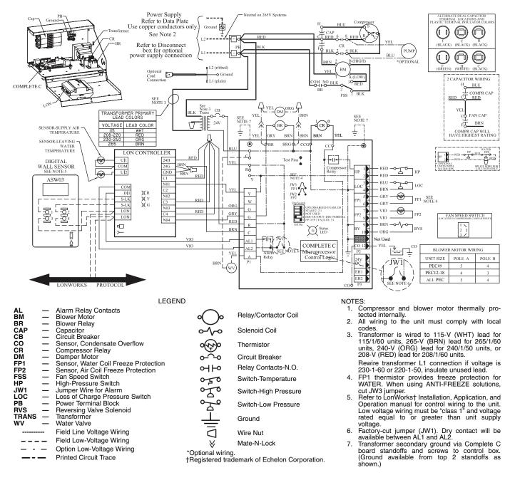
Fig. 18 — 50PEC Unit with Complete C and LON Controllers
